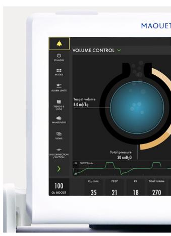
Servo Compass visualizes the volume and pressure of each breath in relation to set targets.
